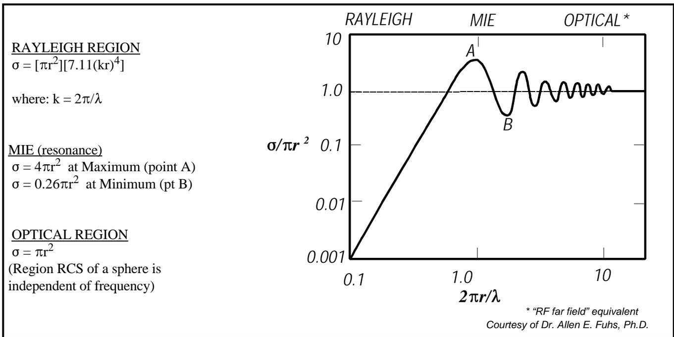
**Figure 7.** Radar Cross Section of a Sphere
