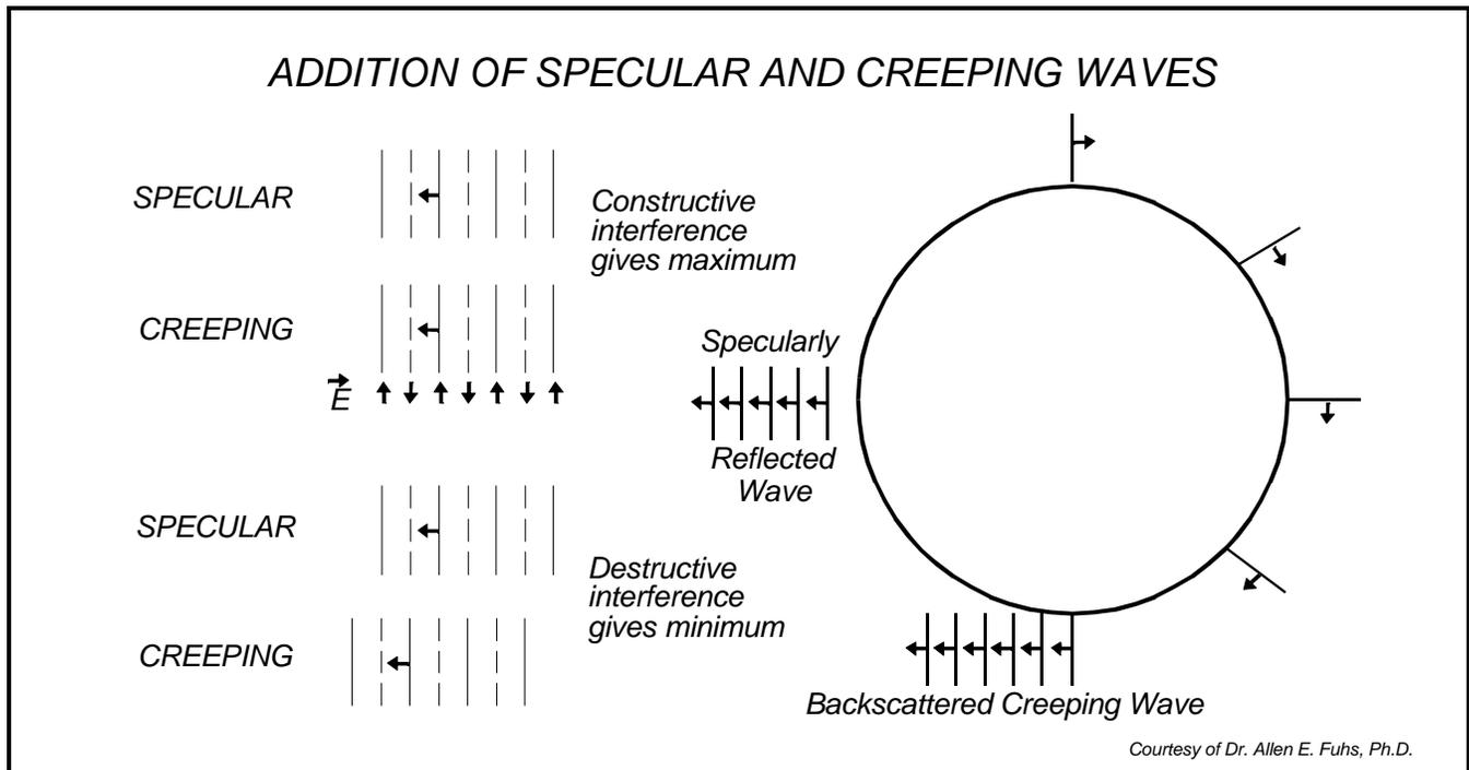
**Figure 8.** Addition of Specular and Creeping Waves
